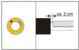
Install the copper wire (the auxiliary or signal wire) in 3 wire holders that ensure the correct distance to the steel pipe.
