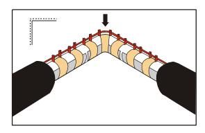
Place the tape so the felt is not pressed against the ends.
