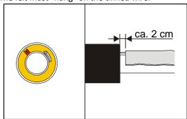
Apply enough wire holders to the signal wire so that the wire cannot be pressed against the steel pipe.
