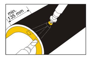
Drill 2 dia. 17 mm holes in to the conical hole. Remove surplus foam and dirt before installing the cable.
