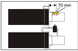
The wire from the connecting/junction box must face towards the outer casing.
