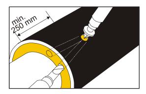
Drill 2 dia. 17 mm holes in to the conical hole from the foam end.
