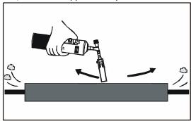
On the finished shrink tube, mastic must be visible at the ends.
