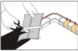
Check that both the steel pipe and the felt are dry during installation.
