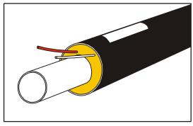
At each joint there must only be one pipe label and it must face upward (12 o'clock position) In the surveillance system the alarm wires are placed at the top of the pipe in order to achieve:
