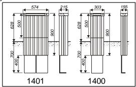
To avoid moisture ingress fill the lower third of the cabinet with styropor balls.
