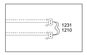
Use long earth connections, part no. 1201 (10 pcs.) so the box is raised above the insulation.
