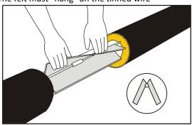
The installation is correct if there are a couple of cm between felt and insulation.
