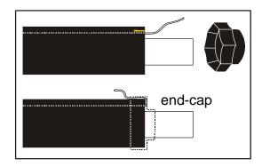
Weld the earth connection on 70 mm from the outer casing end.
